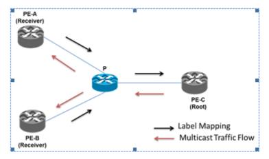
Figure 2: mLDP Setup with root, receivers and P router holding the P2MP state
